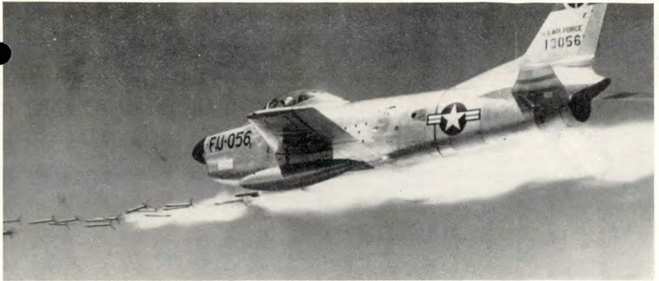
Formation flying, gunnery and high angles of attack can result in compressor stalls.
