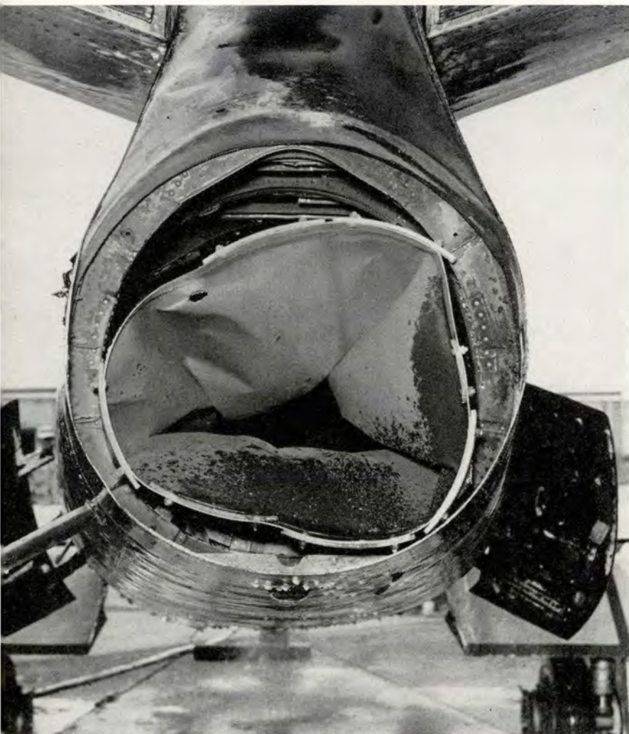
If you need convincing that compressor stall can be serious and cause extensive damage, check the photos. All three pictures are of the same F-86F aircraft.
